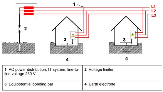
Figure ZC.1 - IT power distribution system in Norway
